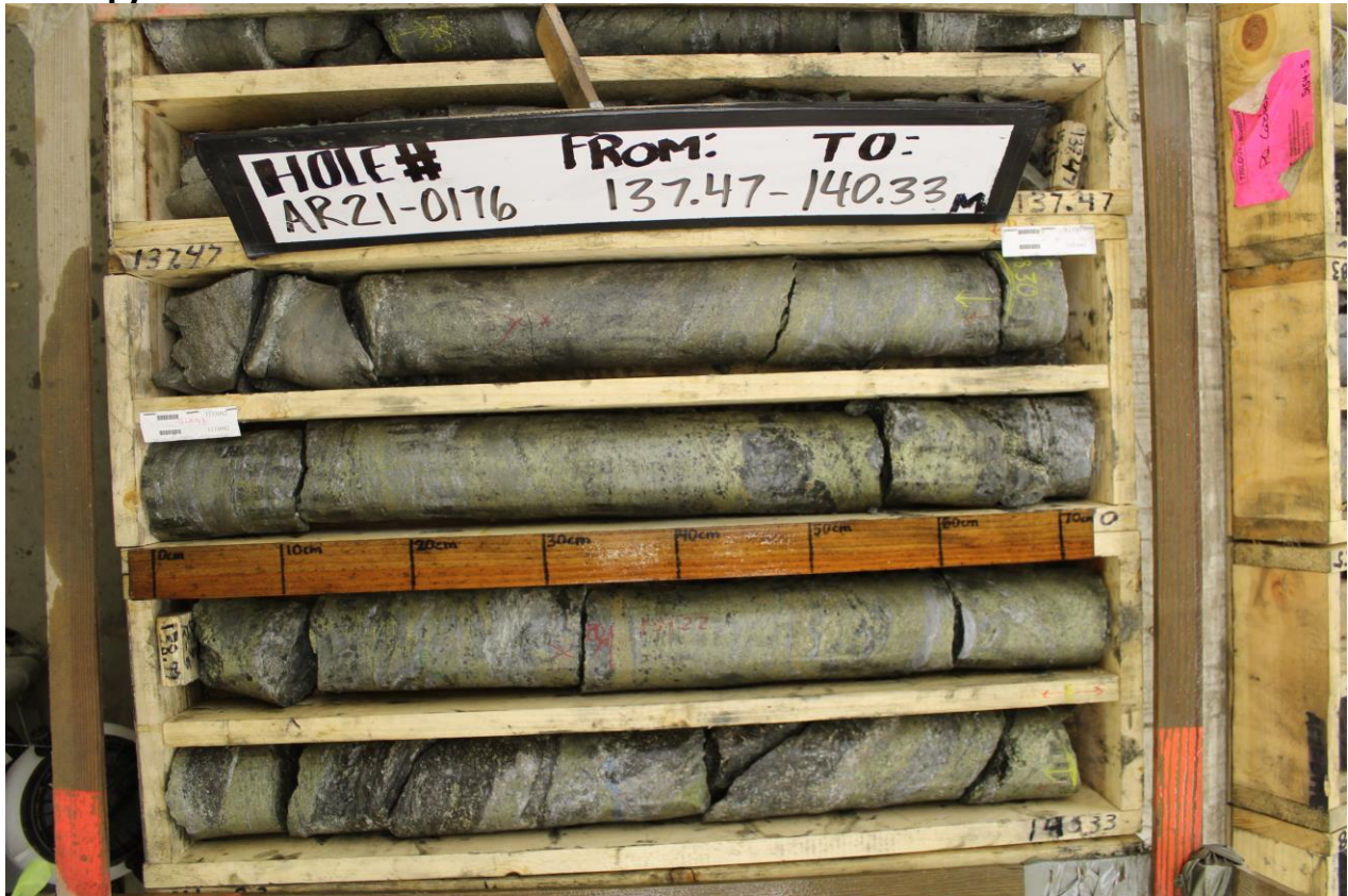
Figure 3. Photo of drill core from Hole AR21-0176 showing massive to semi-massive chalcopyrite.
